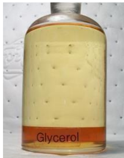
Figure 41 Bottle of biodiesel (top layer) and glycerol (bottom layer)
